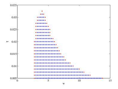
FIGURE 2. Combinations of  $\tau$  and w that ensure stabilization. Experimental results.
